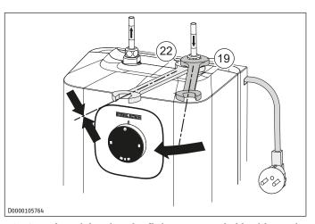
NOTICE: When tightening the fittings, counterhold with a suitable spanner.
