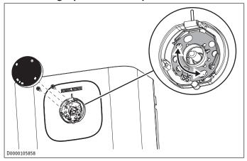
Placing the limiting ring behind the temperature selector allows you to limit the setting range of the temperature selector to a specific maximum temperature.
